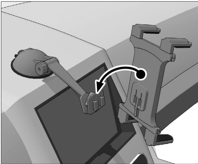
**2** Mount tablet by pushing down on bottom legs; adjust mount & support legs as necessary.
